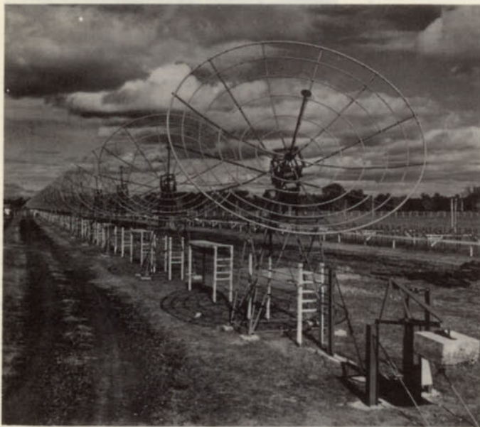
Fig 2.2 The radiophysics division of Australia's Commonwealth Scientific and Industrial Research Organisation has produced this radio telescope designed specifically to pinpoint and photograph small areas of the sun. It is able to focus on less than one per cent. of the sun, and show 10 000 times more detail than a first-class radar set. The telescope was invented by Dr. Wilbur Christiansen, of the radiophysics division of C.S.I.R.O., Sydney, and was set up in a site about 30 miles from Sydney.
