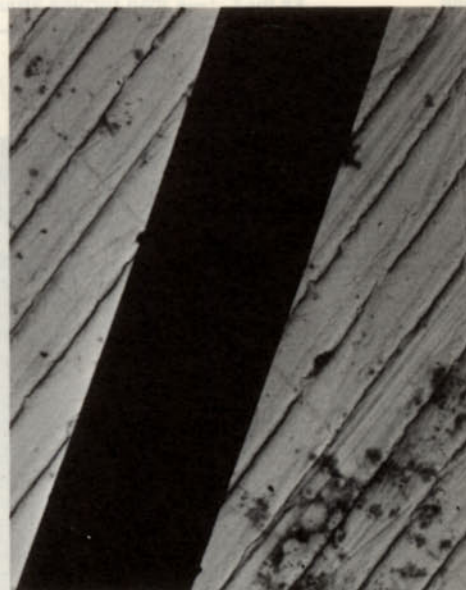
Fig 2.5 This microphotograph of a tungsten wire of nominal diameter 5\mu\text{m} was taken against a grid with 2600 lines/centimetre. What is the degree of magnification? What was the actual diameter of the wire?
